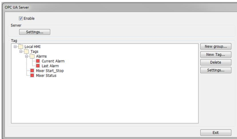
The addresses that can be monitored and controlled are not limited to Local HMI addresses; PLC addresses can be added as well.
