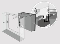
and the provided brackets and screws. Screw Torque: 2.6 ~ 3.9 lbf.in. (For reaching waterproof effect and preventing the panel from being deformed.)
