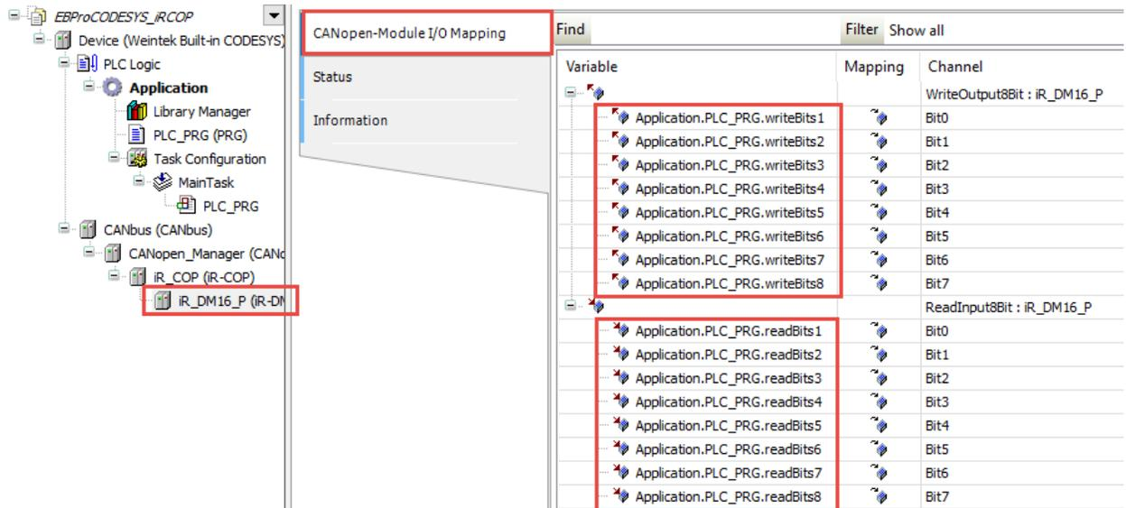
10. Still on the CANopen I/O Mapping tab, set Always update variables to Enabled 2 (always in bus cycle task).
