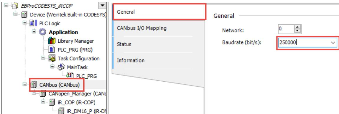
7. To map tags to the CANopen device, first add tags to the PLC\_PRG application. In this example, BOOL tags are used as the only IO module connected to the iR-COP is an iR-DM16-P:
