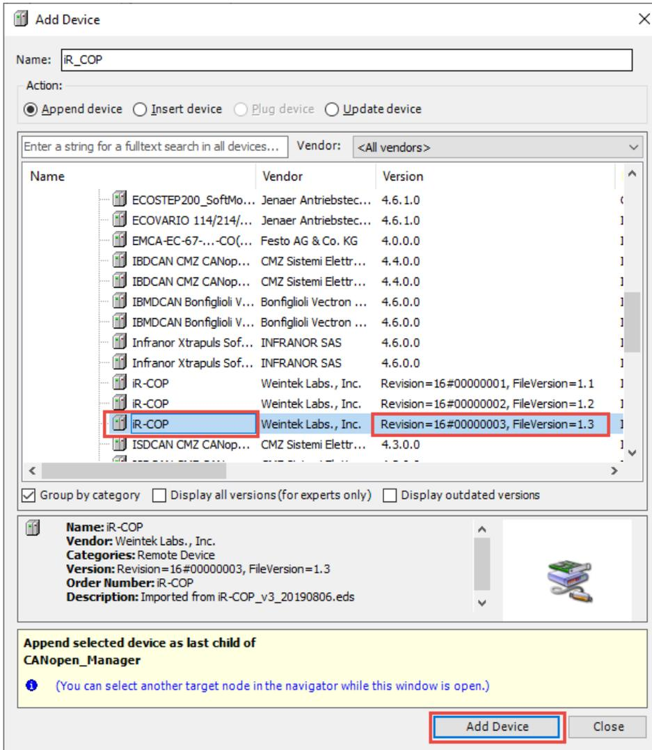
5. Select the newly added iR-COP device, and then in the Add Device window, add each module connected to the iR-COP in the order connected. In this example, we only have an iR-DM16-P connected:
