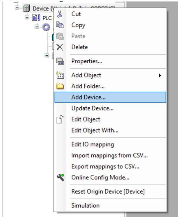
2. In the Add Device window, first check the Display all versions checkbox, and then select Fieldbusses -> CANbus -> CANbus version 3.5.10 and click Add Device:
