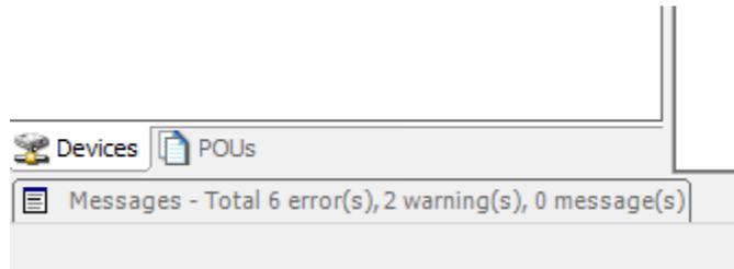
Clicking on this will open the errors and warnings. If there are any errors, and this is the first CODESYS project created, build errors are likely due to missing libraries. Open the errors and double click one to open the Library Manager:
