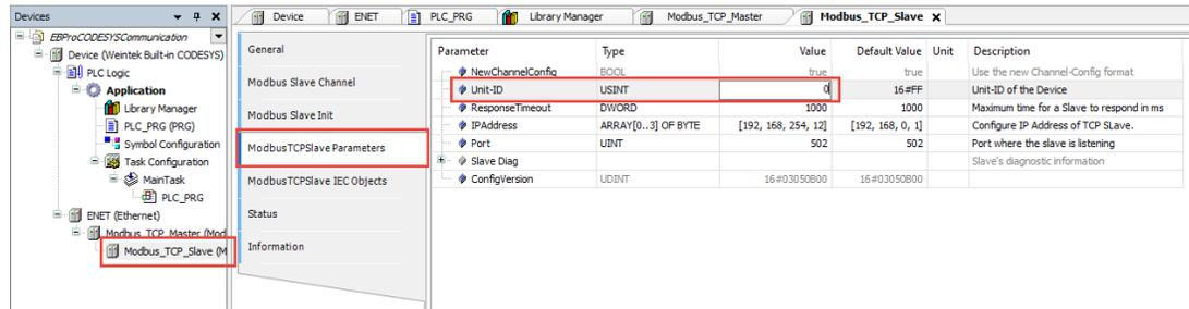
10. To add a tag to the Modbus device, go to the Modbus Slave Channel tab and click Add Channel to open the Modbus Channel window. Select the access type to match the data type of the tag. In this case, a bool-type tag is being added, so the Read Discrete Input type is used:
